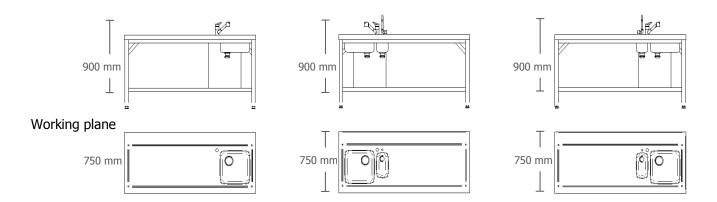
Codes in this page refer to working planes made of AISI 304 stainless steel. On demand are available working planes with the same configurations made of AISI316 stainless steel or coated with melamine resin (smooth plane)
