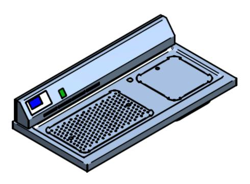
The plane is made entirely of AISI 304 stainless steel, with smooth surfaces and rounded edges. The characteristic cradle profile ensures a good containment of liquids that might otherwise accidentally spill on the floor.
